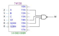
We have seen in class that the decoder generates all possible minterms. Therefore, a decoder can be used to implement any SOP by OR-ing appropriate outputs (minterms) of the decoder. In this case, the outputs of the decoder are active-LOWs. So, instead of the OR gate, we need a negative-OR gate where the "negative" is needed to cancel the bubbles on the outputs of the decoder. Of course, negative-OR gate is the same as the NAND gate.
