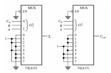
In class, we have seen that the output of a MUX is a weighted sum (OR) of all minterms where the weights are the inputs. Here we feed 1 in the inputs that correspond to the minterms that we want.
