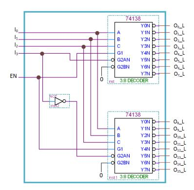
We connect the EN line to G1 of both decoders. Because G1 is active-HIGH. EN = 1 will enable both decoders and EN = 0 will disable both decoders.
